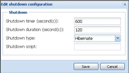
**Figure 110. Edit Shutdown Configuration Dialog Box**
