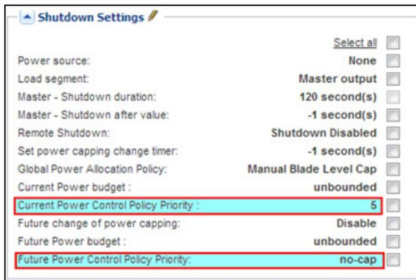
Figure 146. Shutdown Settings-Current Power Default Setting (Priority 5)
