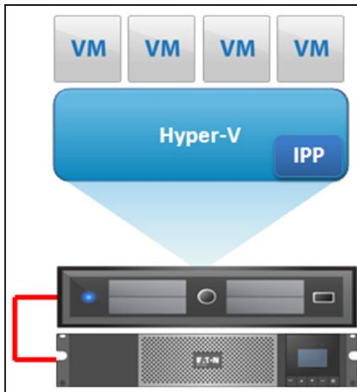
**Figure 83. Eaton IPP Running on Hyper-V to Protect Hyper-V**
