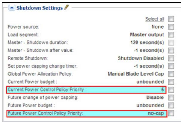
Figure 147. Shutdown Settings-Current Power Not Set Due to No-Cap Service Profile
