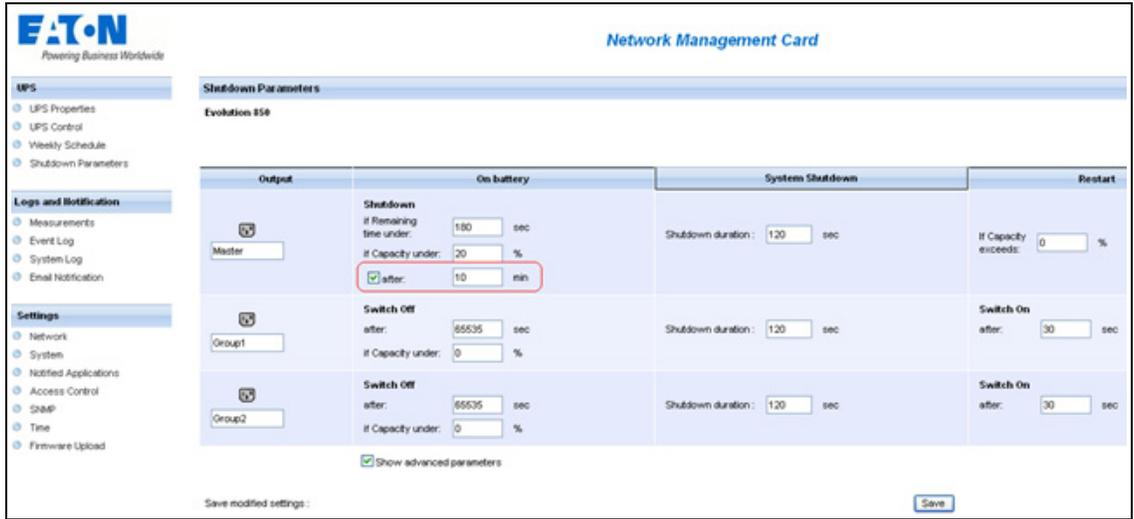
Figure 111. Network Management Card Shutdown Parameters
