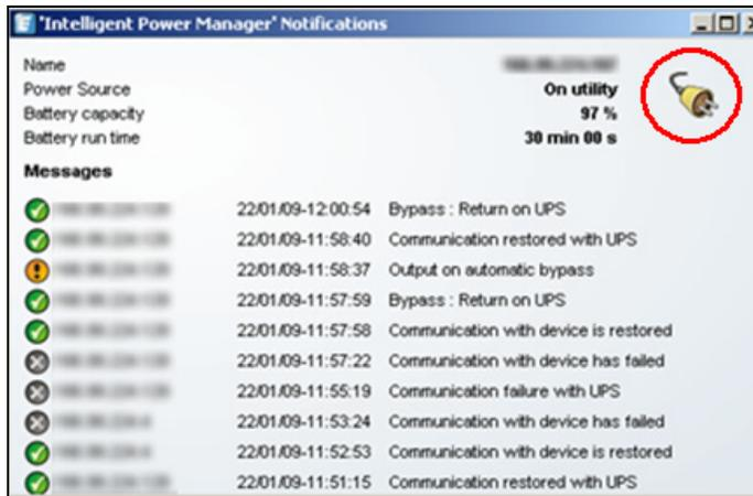
**Figure 35. Alarm Notification Box with System Tray Icon**
