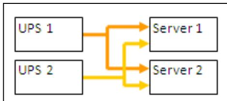
**Figure 98. Redundant Supplies**
