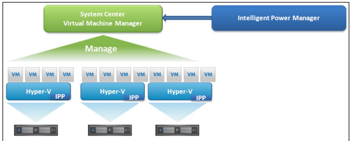
Figure 84. Eaton IPM Connected to SCVMM to Protect Microsoft Virtual Infrastructure
