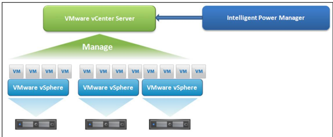
Figure 77. Eaton IPM Connected to vCenter to Protect VMware Infrastructure
