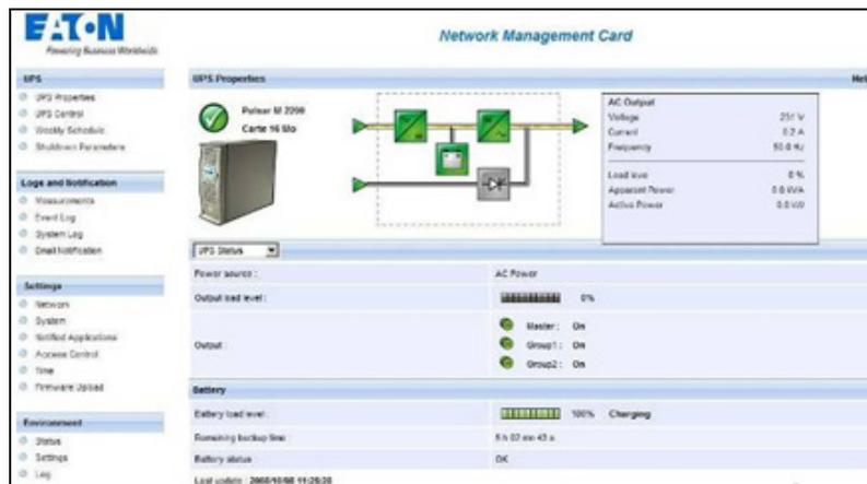
The screenshot shows the Eaton Network Management Card web interface. The top section displays 'UPS Properties' for a 'Purifier M2 2000' card. It includes a diagram of the power flow and a table of AC Output parameters:
