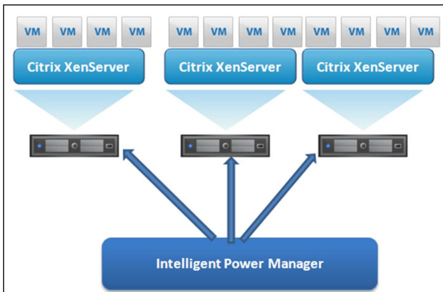
**Figure 89. Eaton IPM Connected To XenServer to protect the XenServers**
