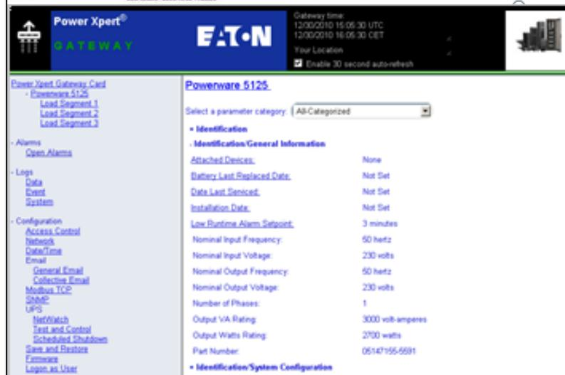
The screenshot shows the Eaton Power Xpert Gateway web interface. The top section displays 'Power Xpert Gateway' and 'EATON'. The 'Gateway Time' is '12/02/2010 16:06:30 UTC' and '12/02/2010 16:06:30 CEST'. The 'Your Location' is 'Enable 30 second auto-refresh'. The main content area shows 'Powerware 5125' configuration. A dropdown menu is set to 'All-Categorized'. The 'Identification' section includes 'General Information' and 'System Configuration'.
