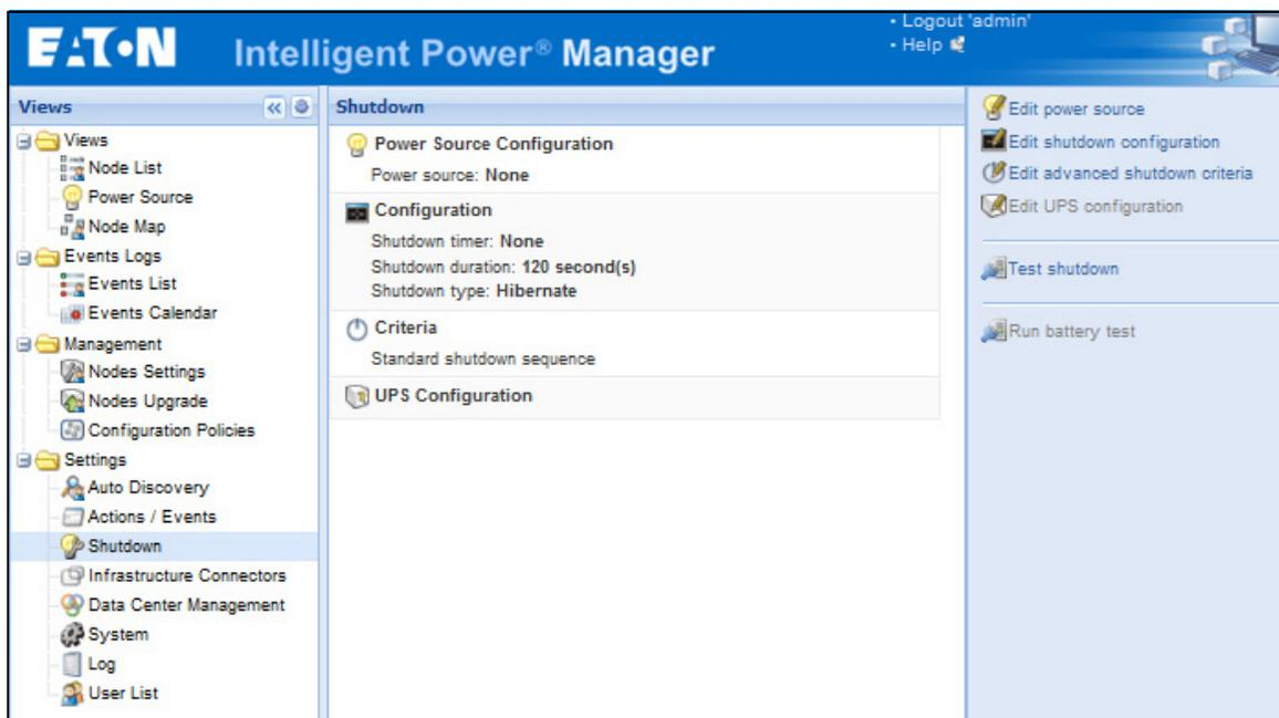
Figure 6. Shutdown Displays in the Settings Menu Hierarchy
