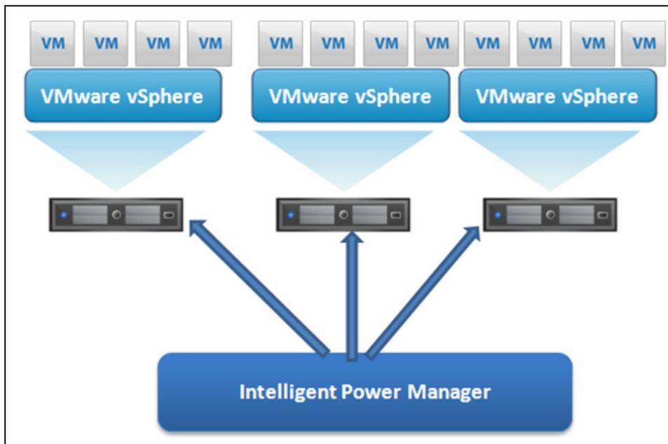
Figure 78. Eaton IPM Connected to ESX/ESXi to Protect VMware Infrastructure (Without vCenter)
