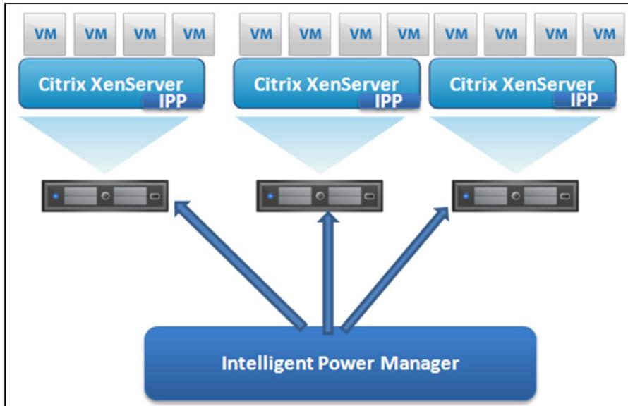
**Figure 88. Eaton IPM Connected to XenServers (Triggers XenMotion and Eaton IPP Running on XenServer Infrastructure)**
